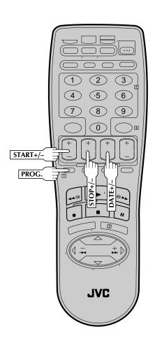
You can directly program the VCR's timer to record up to 8 shows, as far as a year in advance. Remember, the clock must be set before you can program the timer ( pp. 8 or 11).
